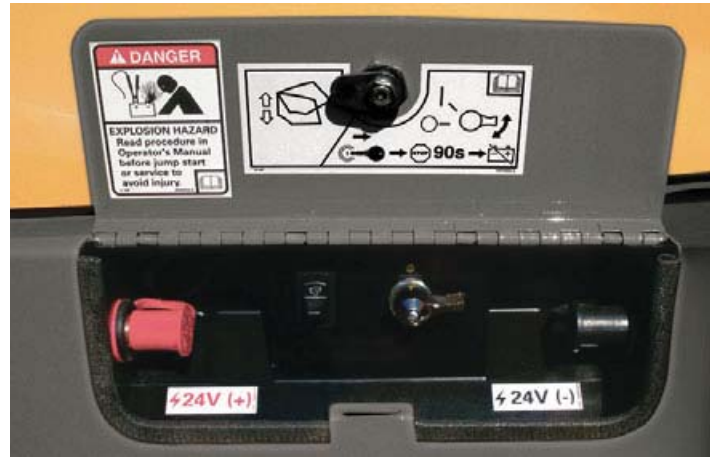
Hood opening and battery on/off switches. In case of flat battery, hood can be opened externally with Remote jump start
